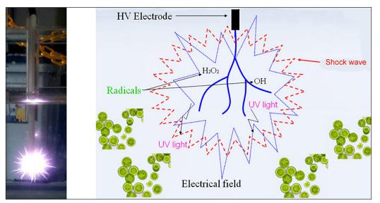
Fig. 4. The discharge phenomena in the water
