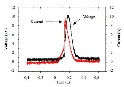
Fig. 3. The waveforms of the applied voltage to and the discharge current during discharge
