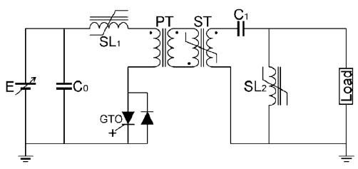
Fig. 1. A diagram of the circuit of the pulse discharge
